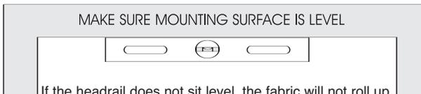
If the headrail does not sit level, the fabric will not roll up evenly which could damage the edges of the shading fabric. Use shims if necessary to level brackets.
