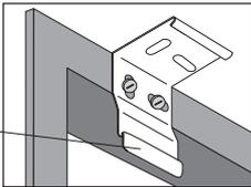
For inside or ceiling mounts, use the top bracket holes.
