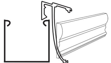
Push valance clip down over front of headrail. Insert the top of edge of the valance (or slat) into the clip then press the bottom into place.
