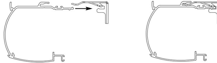
Push the rail back until it is fully engaged.
