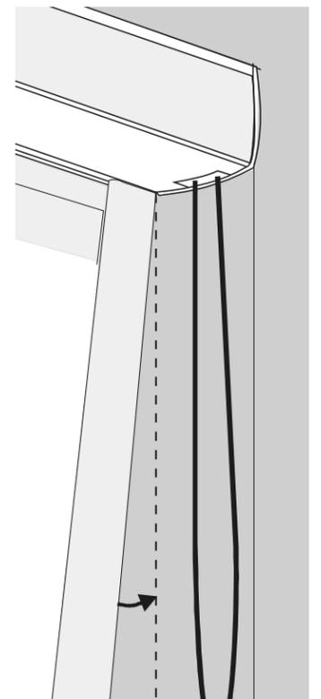
Slide the fabric into the track but keep the track away from the edge of the window so that the exposed adhesive does not touch the wall.
