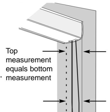
Mark the bottom of window at the same point as the top measurement.
