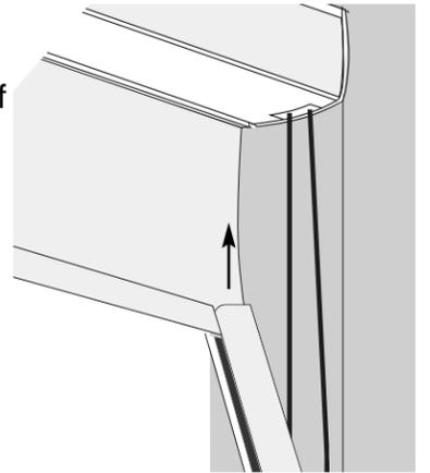
The inner black track should be even with the bottom of the outer track.
