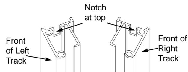
Slide the fabric lip into the track. Slide the track up so that the top of the track goes into the slot on the headrail.
