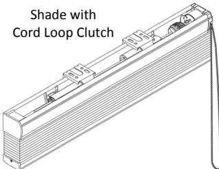
Position the first two installation brackets so that they are approximately 2" in from the end of the headrail. If a third bracket is included, center it between the outer brackets. Wide shades may include up to 8 brackets. In these cases, space the additional brackets evenly, not more than 25" apart. Mark the brackets for mounting hole locations, making sure they are square and equally spaced. For outside mount installations, use a level to check for levelness.
