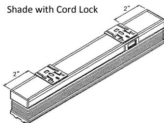
Position the first two installation brackets so that they are approximately 2" in from the end of the headrail. If a third bracket is included, center it between the outer brackets. Wide shades may include up to 8 brackets. In these cases, space the additional brackets evenly, not more than 25" apart. Mark the brackets for mounting hole locations, making sure they are square and equally spaced. For outside mount installations, use a level to check for levelness.
