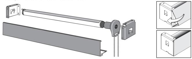
2. INSTALL THE SHADE. Push the clutch straight onto the blade of its bracket. The bottom of the clutch should always point straight down, as shown above. Lower the lug of the end plug onto the "V" of its bracket. The roller should fit in the brackets securely, with just a little play.
