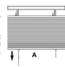
If the cord needs to be longer, slide the bottom end of the cord up into the wedge and slide the wedge down to take up slack.
